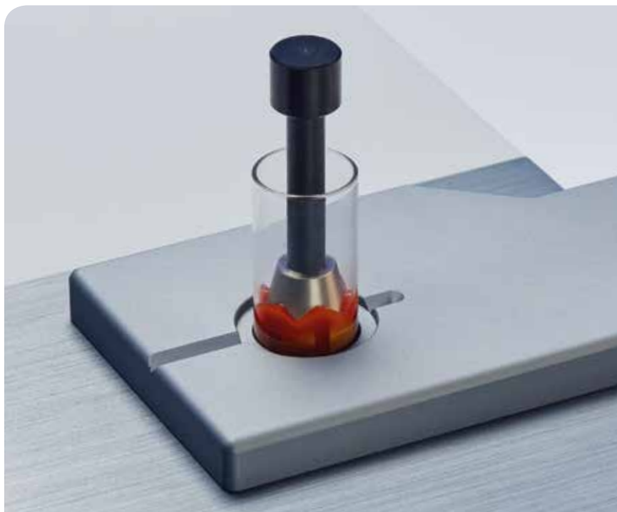
Transfection measurement of ketchup in a 22mm vial on the integrating sphere of the MPA II
