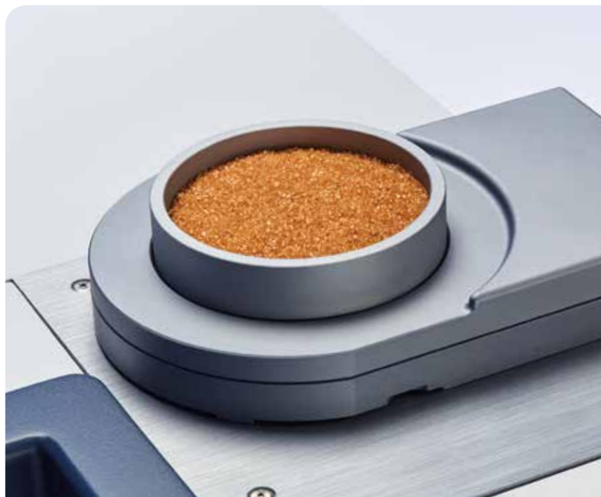
Measurement of raw sugar in a Quartz cup on the integrating sphere of an MPA II spectrometer
