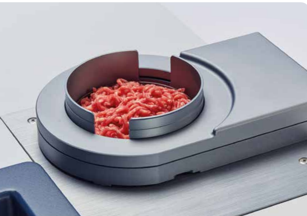
Measurement of minced meat in a polystyrene Petri dish on the integrating sphere of an MPA II spectrometer
