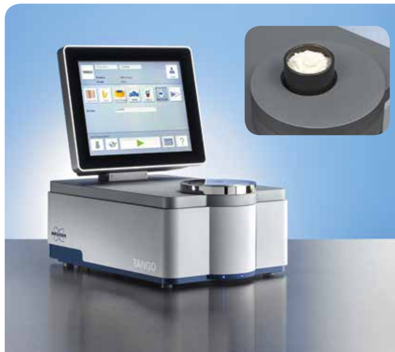
Measurement of flour in a quartz glass cup on the integrating sphere of the TANGO-R FT-NIR spectrometer
