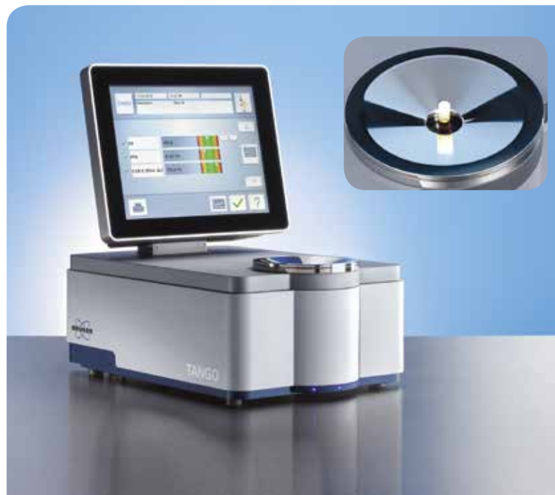
Measurement of edible oils in an 8mm vial in the sample compartment of the TANGO-T FT-NIR spectrometer
